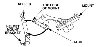
Figure 2-24. Installation of Helmet Mount.
